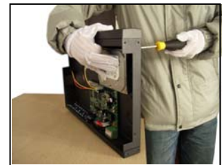
③ fix the screw of hard disk
