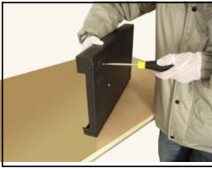
④ fix the screw of hard disk
