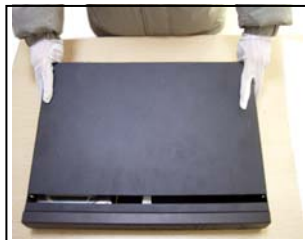
② disassemble the cover
